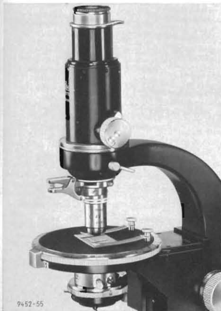
SM-POL with photographic-Pol-tube O 14 and objective centring clutch
